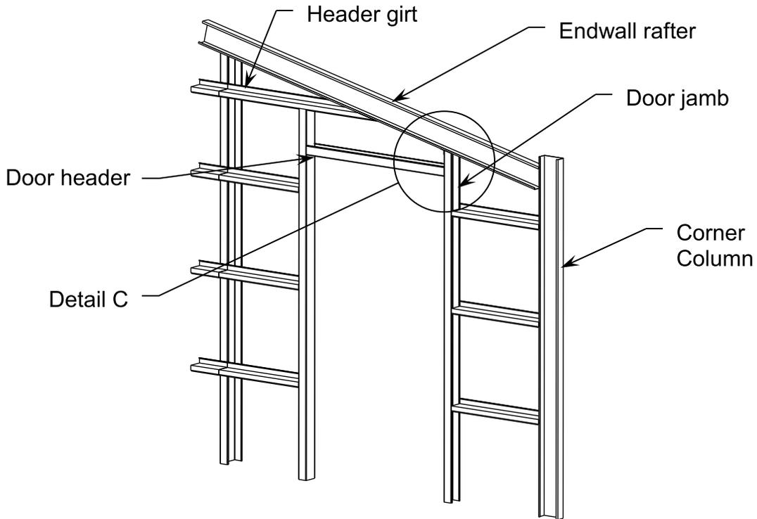
When this is the case, the door jamb will be installed as shown below in Detail C. Note that the top of the door jamb will need to be coped to fit the bottom of the rafter, and the correct sized girt clip that connects the door jamb to the rafter will need to be bent to fit as well. Note that the door jamb base will be installed as shown and described above, as per engineering plans.
